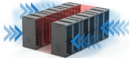
Hot aisle containment
